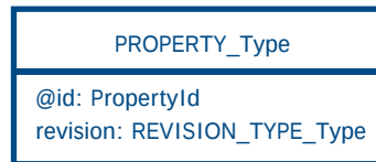
Figure 5 – UML-like representation of XML attributes and simple type elements
